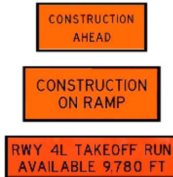
The airport operator may choose to introduce temporary construction signs with a black message on an orange background.
